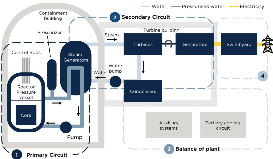
Note: Diagram based on a Pressurized Water reactor plant (PWR), but also applicable to Pressurized Heavy-Water Reactors (PHWR) and Boiling Water Reactors (BWR)
